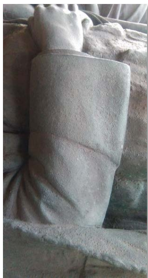
The Founder's Tomb – the surfaces of the bronzes are covered with pustules, which appears to be a sign of widespread bronze disease
